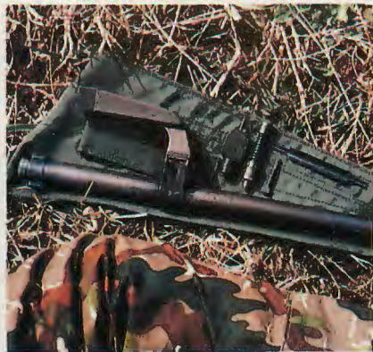
UPPER LEFT: Weapon's rear sight is adjustable to 1,000 meters. ABOVE: MG82 barrels feature hard-chromed bores and chambers, are available with either 1:7-inch or 1:12-inch twist. LEFT: Barrel may be changed within a few seconds. Note carrying handle attached to it.
